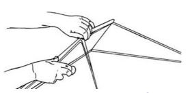
With fingers in the hole, raise side 4 into position. The left hand will have to prise back side 3 a little to enable the location point to be aligned on the corner joint between sides 3 and 4, the same is done for corner joint 4 and 1.
