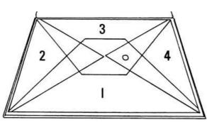
Zip open folder on a bench top. Have top spring clip to hand. Raise sides in sequence as shown. Assemble corner joints with location points on corners.
