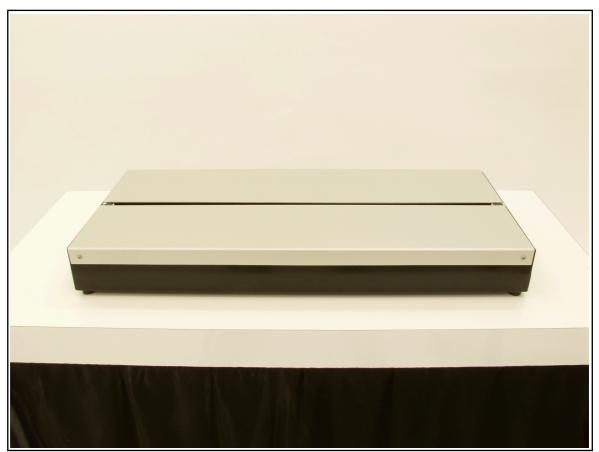
The **RH Acrylic Folder** is designed for heating acrylic sheet such as  $Perspex^{TM}$ , to make display stands for collection objects.
